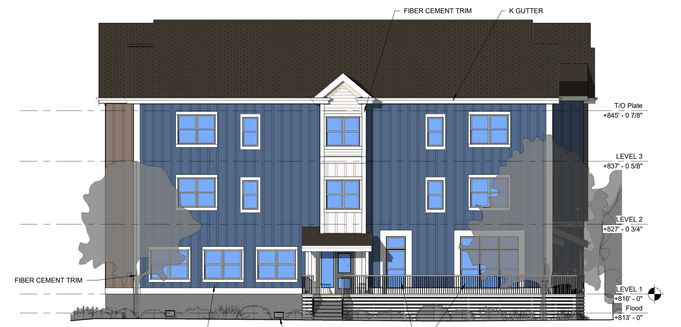
2 EXTERIOR ELEVATION - NORTH 1/8" = 1'-0"
