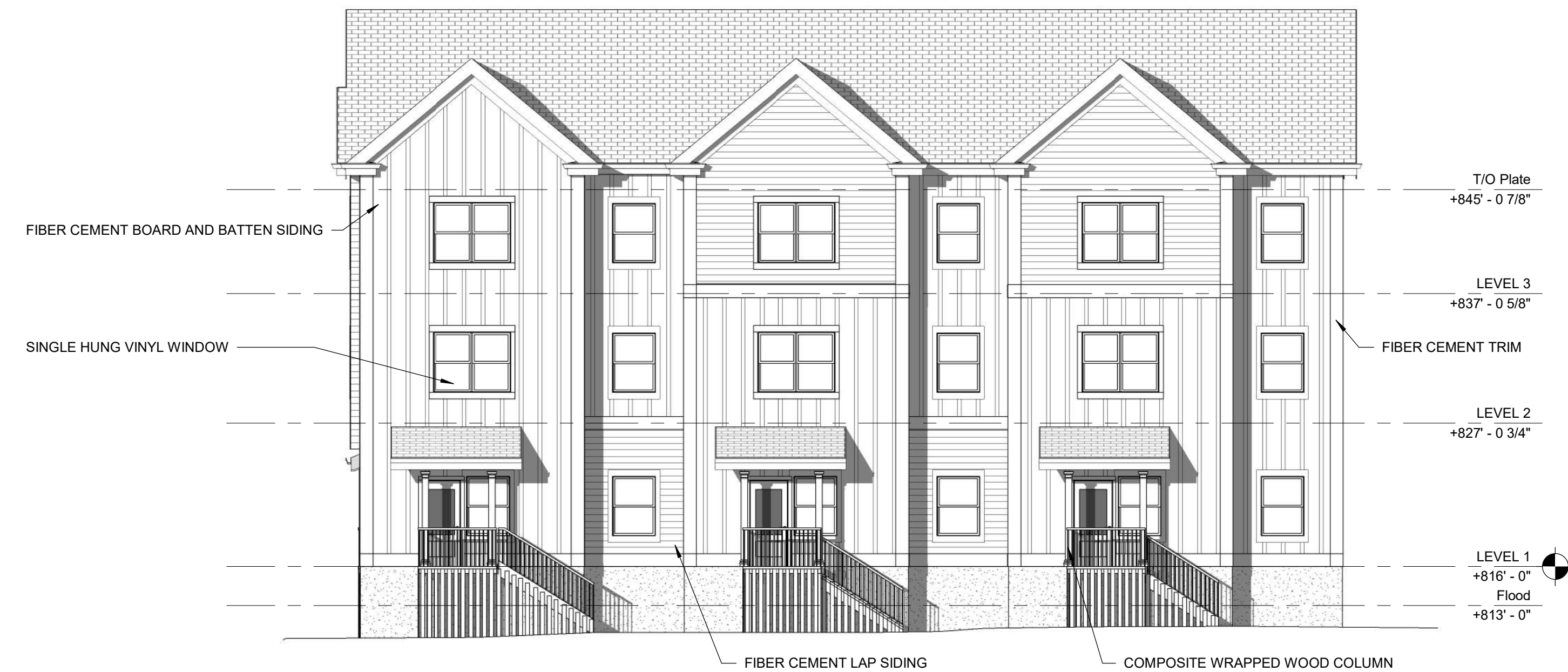
3 EXTERIOR ELEVATION - SOUTH (TEMPLE ST) 1/8" = 1'-0"
